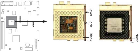
SP98-N ZIF Socket 7 with Pentium MMX Processor
