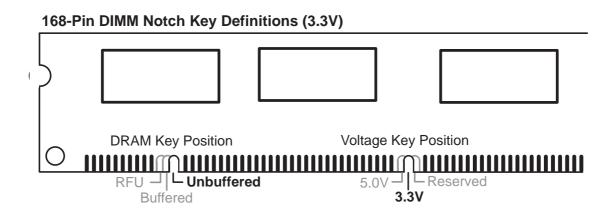
The notch on the DIMM module will shift between left, center, or right to identify the type and also to prevent the wrong type to be inserted into the DIMM slot on the motherboard. You must ask your retailer for the specifications before purchasing. Four clock signals are supported on this motherboard.
