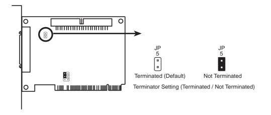
Decide whether or not you need to terminate the ASUS PCI-SC200 based on its position in the SCSI chain. Only the devices at each end of the chain need to be terminated. If you have **only** internal or **only** external devices connected to the ASUS PCI-SC200, then you **must** terminate the ASUS PCI-SC200. If you have **both** internal and external devices connected, you **must not** terminate the card. See the following examples which illustrate this concept.
