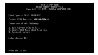
**IMPORTANT!** If "unknown" is displayed after **Flash Type --**, the memory chip is either not programmable or is not supported with the PnP BIOS and therefore cannot be programmed by the Flash Memory Writer utility.
