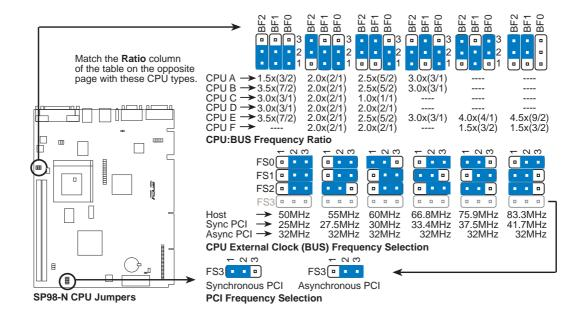
**WARNING!** Do not overclock your processor. Overclocking can cause undue stress on the CPU and motherboard. It may result in a slower speed or other unpredictable outcomes. The table on the following page shows the approved CPUs and their settings.
