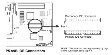
**TIP:** You may configure two hard disks to be both Masters using one ribbon cable on the primary IDE connector and another ribbon cable on the secondary IDE connector. You may install one operating system on an IDE drive and another on a SCSI drive and select the boot disk through BIOS Features Setup.
