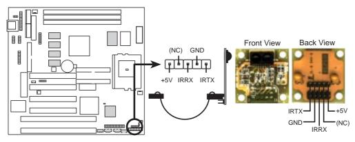
P5-99B Infrared Module Connector
