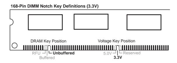
The notches on the DIMM will shift between left, center, or right to identify the type and also to prevent the wrong type from being inserted into the DIMM slot on the motherboard. You must tell your retailer the correct DIMM type before purchasing. This motherboard supports four clock signals.
