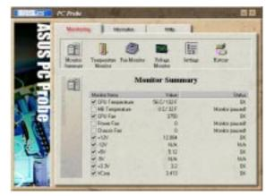
Temperature Monitor Shows the PC's temperature.
