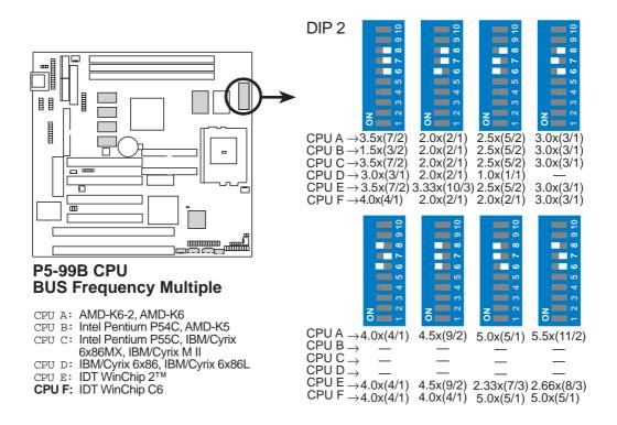
See next page for a table of the CPU BUS Frequency and CPU Core:BUS Frequency Multiple Settings of supported CPUs.
