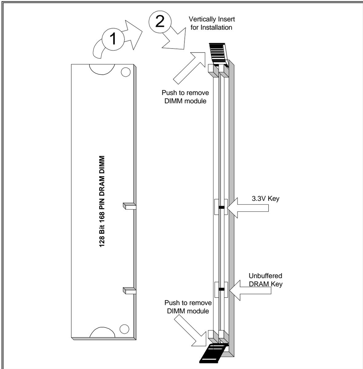
**168-Pin SDRAM Module Installation Diagram**
