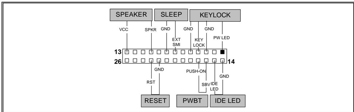
**The Onboard Function Connector Pin Out**
