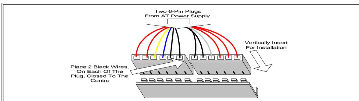
AT Power Connector Installation
