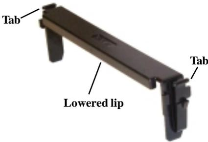
**Make sure the lower lip of the overhead clip is oriented towards the opposite side of the CPU fan (see Figure I left).**
