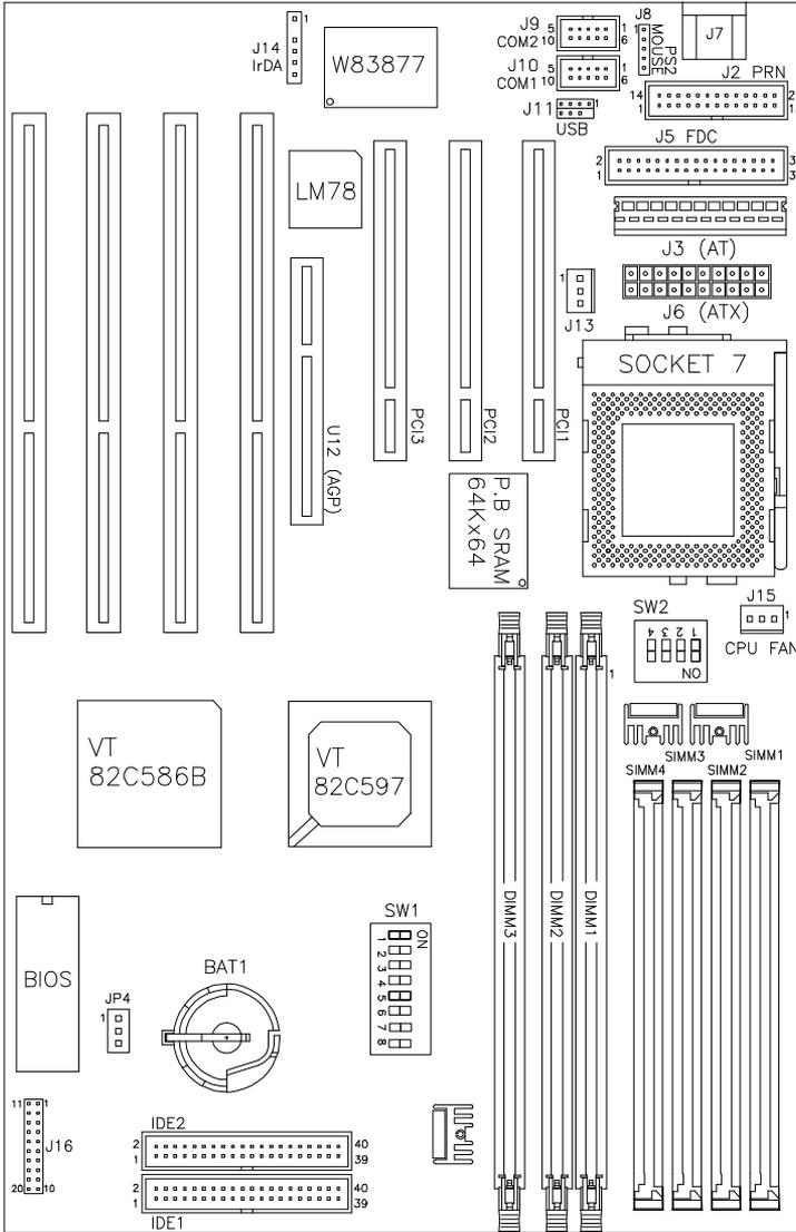
**Figure 2: Jumper Locations of the AI5VG**
