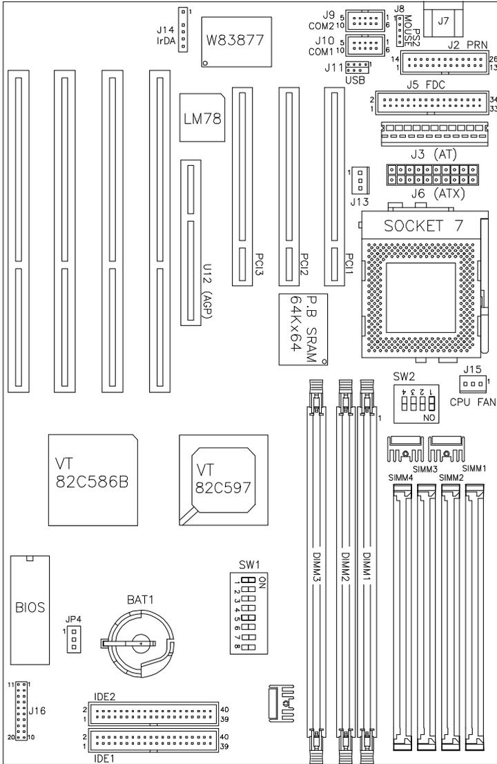
Figure 1: Layout of the AI5VG Motherboard
