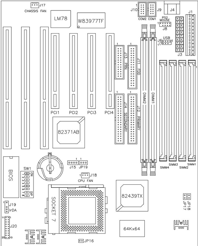
Figure 2: Jumper Location of the AI5TT
