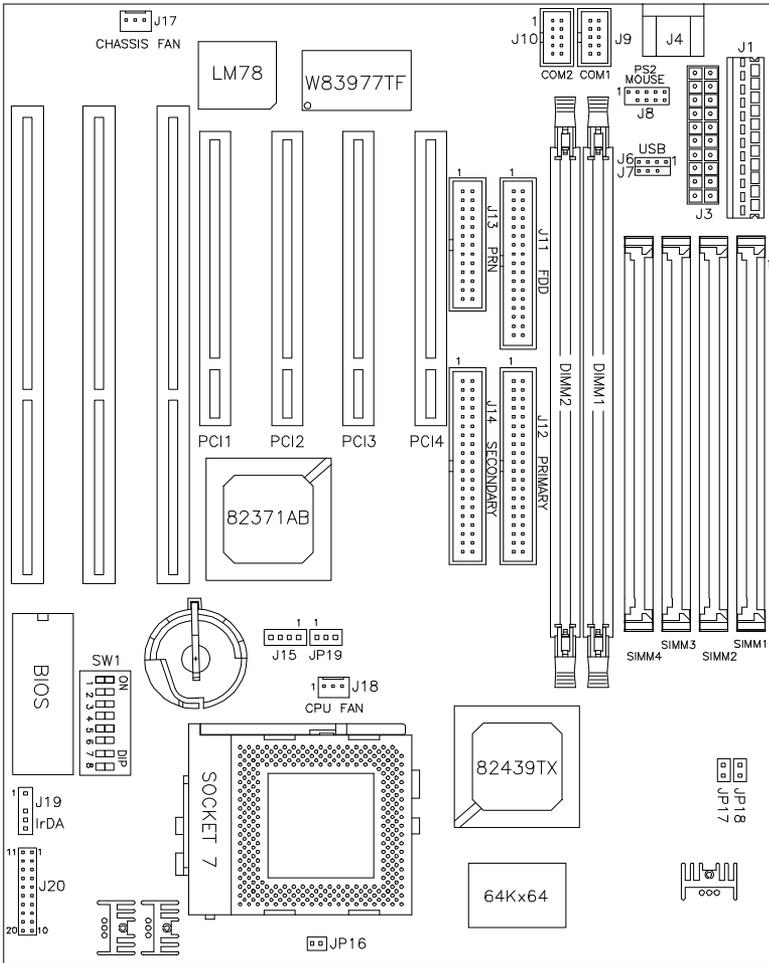
Figure 1: Layout of the AI5TT Motherboard
