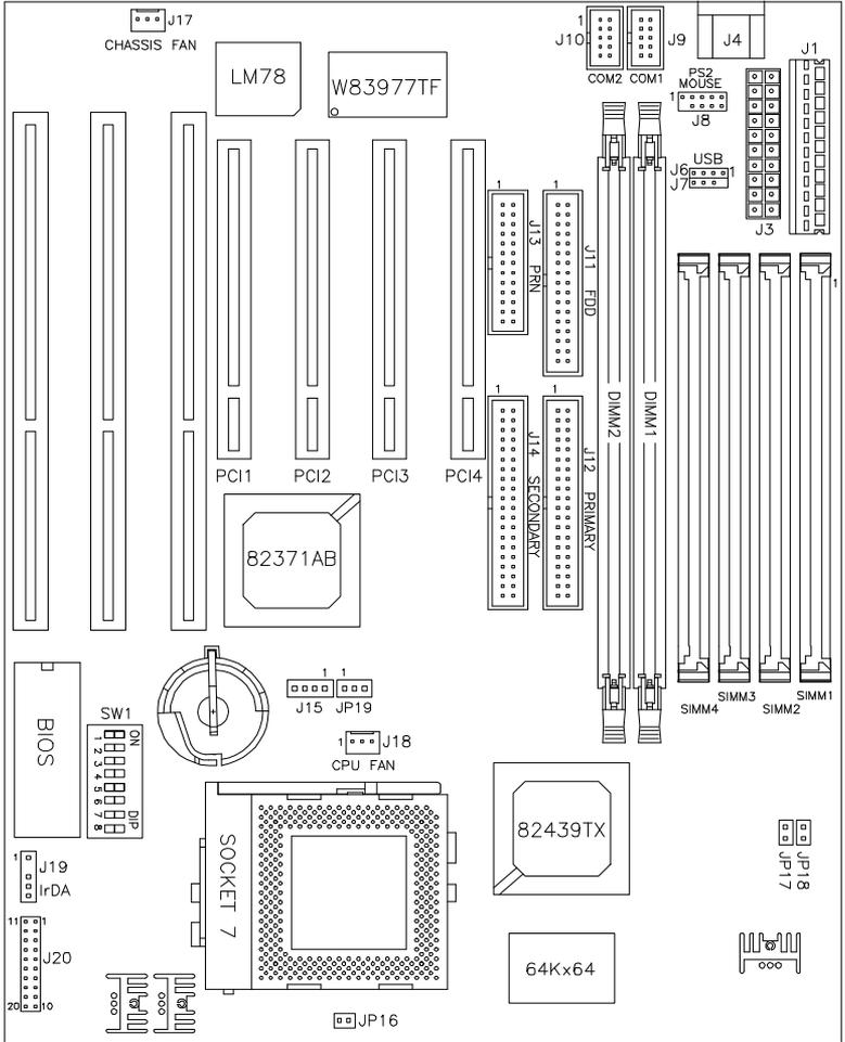
**Figure 3: Connector Locations of the AI5TT**
