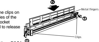
4 Insert the DIMM vertically with its metal fingers aligned with the socket's grooved slot.
