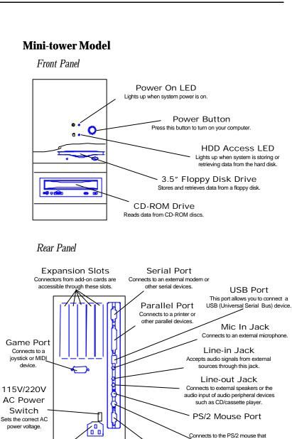
PS/2 Keyboard VGA Port AC Power In Connects to an SVGA//VGA monitor. The female end (with holes) of the power Connects to the PS/2 keyboard that cord is connected to this socket.
