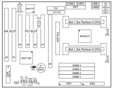
Figure 1–2. Mainboard Default Setting
