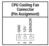
Note: Make sure the pin assignment of our CPU Cooling Fan is matched with this connector before connecting it, otherwise, you may damage either the mainboard or the cooling fan.
