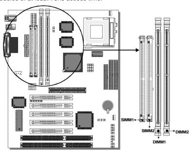
This mainboard supports both EDO and SDRAM types of memory modules.
