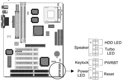
Plug the computer case's front panel devices to the corresponding connectors on the mainboard.
