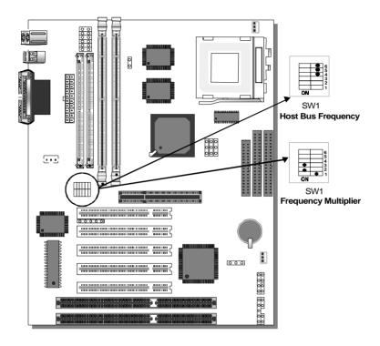
The SY-5EMA mainboard is designed to support most Pentium® class processors currently on the market. Jumpers SW1 is used to configure the mainboard frequency parameters to match the working frequency of your CPU.
