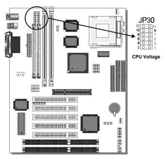
Please verify the correct voltage with your dealer before installation. Use the following tables to set JP30 to the proper "Voltage Value", according to the specifications marked on your CPU: This mainboard comes with pre-configured setting of CPU voltage. However the voltage of your CPU maybe different with the default setting.
