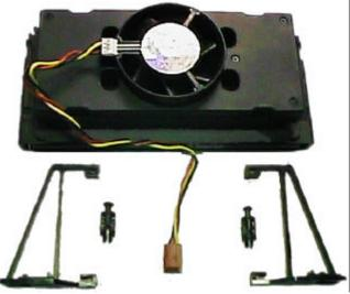
Figure 4:Boxed Pentium® II Processor & Heat sink support
