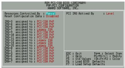
Figure 4.6:PCI Slot Configuration
