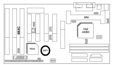
Danger of explosion if battery is incorrectly replaced.
