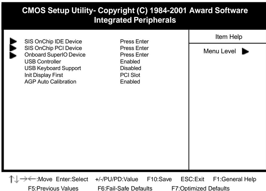
Figure 3-5 Sample of Integrated Peripherals Screen
