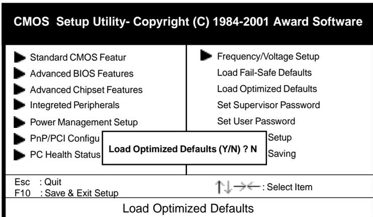
Figure 3-11 Sample of Load Optimized Defaults Screen
