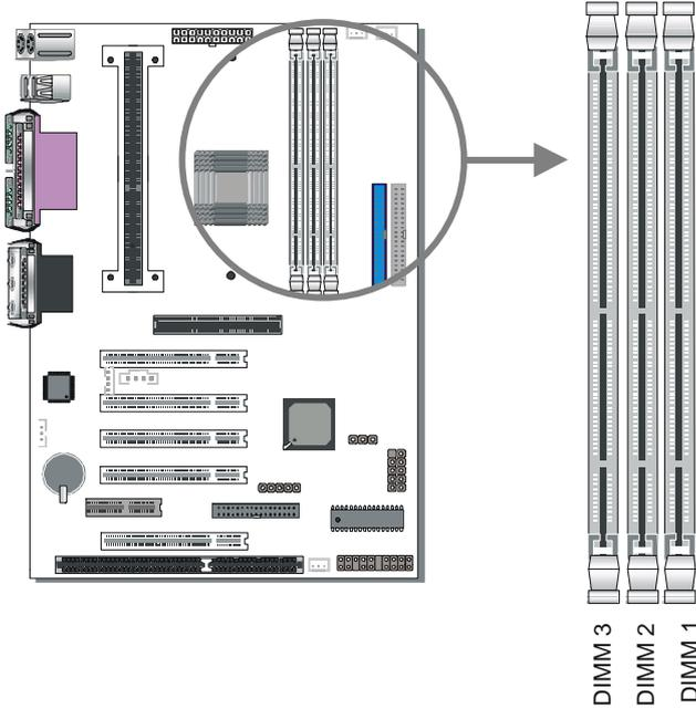
Your board comes with three DIMM sockets, providing support for up to 1.5GB of main memory using unbuffered DIMM modules from 8MB to 512MB. PC100 DIMM module is required on this motherboard.
