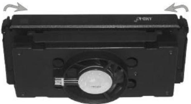
3. Insert the CPU into the retention module. The CPU fits in the CPU slot in only ONE way, do not try to force it in.
