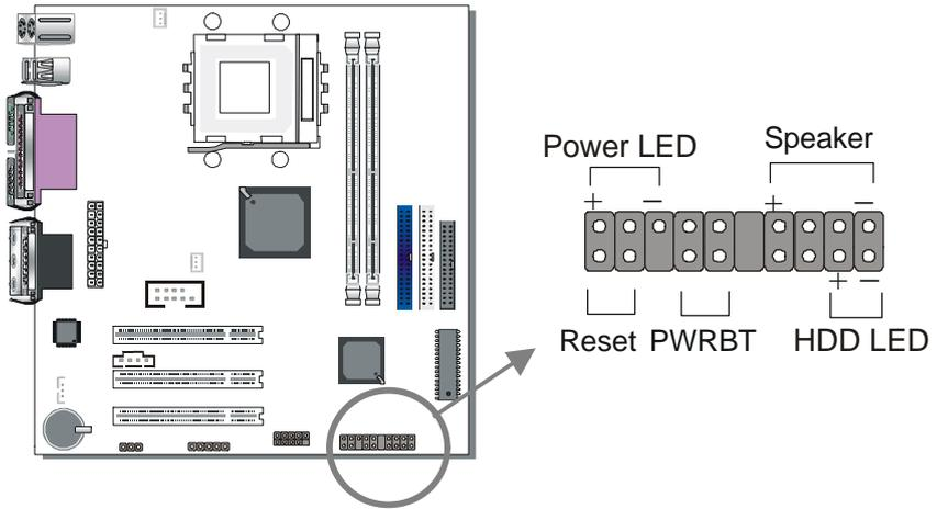
Plug the computer case's front panel devices to the corresponding headers on the Motherboard.
