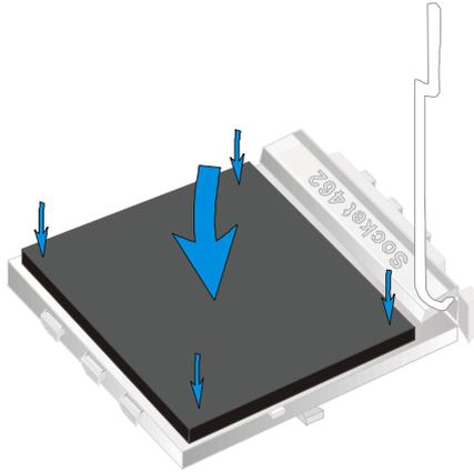
3. Seat the processor in the socket completely and without forcing.
