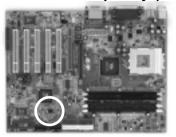
This jumper allows you to select the system bus frequency speed of your CPU. Set the jumper cap to pins 1-2 for 100MHz FSB, set the jumper cap to pins 2-3 for 133MHz FSB.
