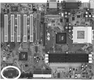
If you enable the UART 2 Mode in BIOS's Integrated Peripherals menu the COM2 port will support IR functions. (See section 3-4)
