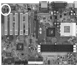
This connector is for Center+Bass speaker output ext. Plug in the optional AC3 Surround Center/Bass and Rear left/right jack extension into this connector. The black colored jack is for surround speaker output and the orange colored jack is for center+bass speaker output.
