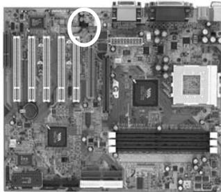
Use the audio cable enclosed with your CD-ROM disk drive to connect the CD-ROM to your mainboard. This will enable your CD-ROM's audio function.
