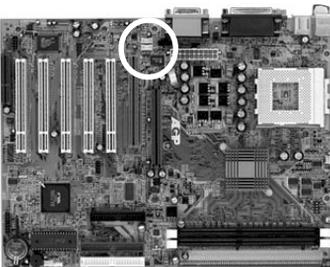
Use the mono audio cable enclosed with your audio device to your mainboard. This will enable mono audio in/out function.
