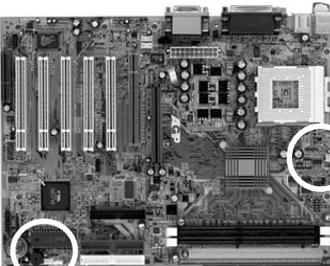
These added connectors allow the fan to draw their power from the mainboard instead of the disk drive connector.
