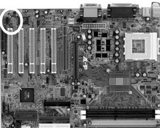
The SPDIF-in/out connector supports the digital audio. This connector must be connected to the cable from an external device. (Ex. 2-channel decoded AC-3 from DVD decoders)
