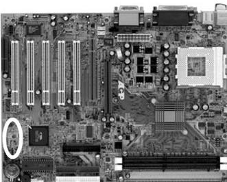
Set the clock ratio according to your processor's specification.
