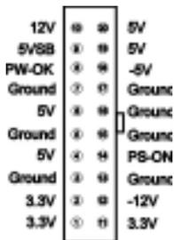
The ATX power supply provides a single 20-pin connector interface which incorporates standard +/-5V, +/-12V, optional 3.3V and Soft-power signals. The Soft-power signal, a 5V trickle supply is continuously supplied when AC power is available. When the system is in the Soft-Off mode, this trickle supply maintains the system in it's minimum power state.
