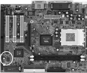
The I<sup>2</sup>C Connector supports the MPEG sound decoder. This connector must be connected to the cable from the MPEG card. This board also contains a connector for optional USB Adaptor (USB2/3). Four USB peripherals or hub devices are able to be connected.
