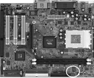
This switch allows you to select between 100MHz FSB or 133MHz FSB frequency speed.
