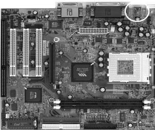
If you want to use a USB keyboard, you must enable the onchip USB & USB keyboard support function in BIOS's Integrated Peripherals menu (See Section 3-4). USB is an open industry standard, providing a simple and inexpensive way to connect up to 125 devices to a single computer port. Keyboards, mice, tablets, digitizers, scanners, bar-code readers, modems, printers and many more can all be used at the same time.
