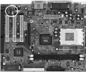
This connector must be connected to the cable from the voice modem card to support modem audio signals.
