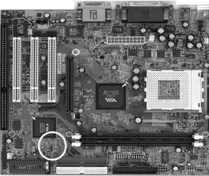
This board supports the chassis instruction monitoring feature of the management extension hardware by means of a mechanical or photo sensor switch attached to the motherboard through this 1x3-pin chassis security header. The mechanical switch is set to open for normal computer operation.
