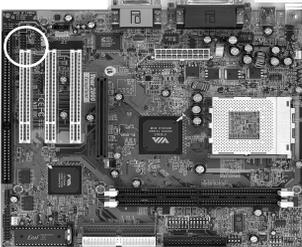
The S/PDIF-Out connector supports the digital audio. This connector must be connected to the cable from an external device. (Ex. 2-channel decoded AC-3 from DVD decoders)
