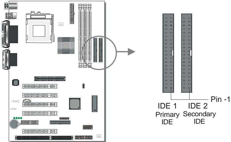
This Motherboard offers two primary and secondary IDE device connectors (IDE1, IDE2). It can support up to four high-speed Ultra DMA 33/66/100HDD or CD-ROM.
