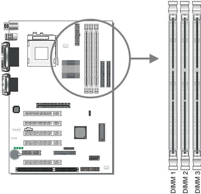
Your board comes with three DIMM sockets, providing support for up to 1.5GB of main memory using unbuffered and registered DIMM modules from 8MB to 512MB. On this motherboard, DRAM speed can be set independent from the CPU front side bus speed. Depending on the DRAM clock speed setting in the BIOS setup (Chapter 3), appropriate memory modules must be used. For 66MHz DRAM speed, use PC66 memory; for 100MHz DRAM speed, use PC100 memory; for 133MHz DRAM speed, use PC133 memory.
