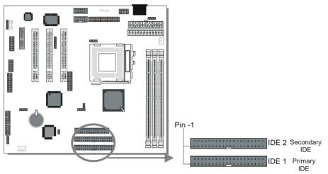
This Motherboard offers two primary and secondary IDE device connectors (IDE1, IDE2). It can support up to four high-speed HDD or CD-ROM.
