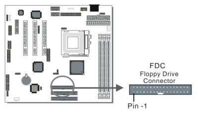
The system supports 5 possible floppy drive types: 720 KB, 1.2 MB, 1.44 MB, 2.88 MB, and LS-120. In addition, this Motherboard supports a 3-mode (720KB/1.2MB/1.44MB) floppy commonly used in Japan. Connect one side of the 34-pin flat cable to the floppy drive and plug the other end to the floppy drive connector on the Motherboard. This Motherboard can support up to 2 floppy drives.
