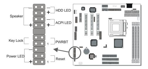
Plug the computer case's front panel devices to the corresponding headers on the Motherboard.
