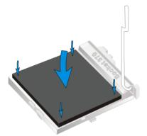
4. Then close the socket handle to secure the CPU in place.
