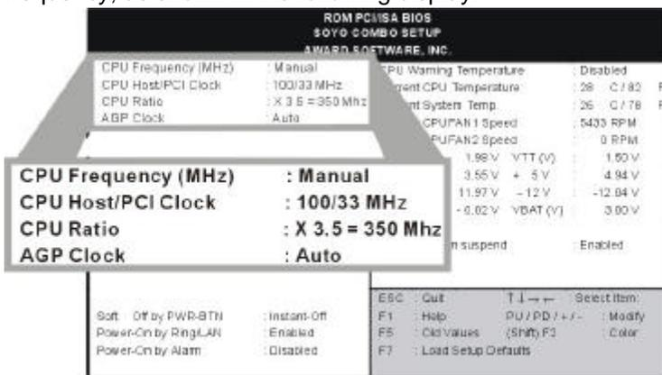
Available [CPU Frequency] settings on your SY-6ZE+ Motherboard are detailed in the following table. If you set this field to [Manual], you are then required to fill in the next two consecutive fields: (1) the CPU Host/PCI Clock, and (2) the CPU Ratio.
