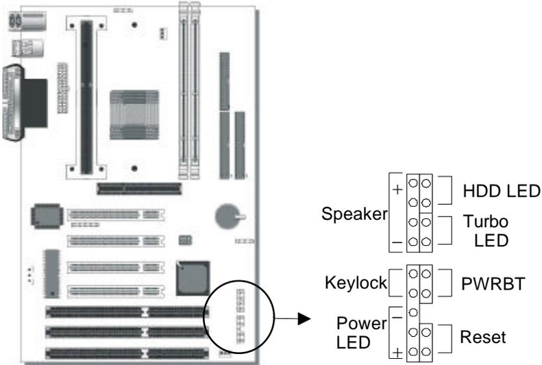
Plug the computer case's front panel devices to the corresponding headers on the Motherboard.
