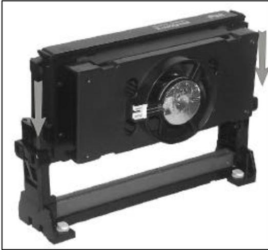
4. After completely inserting the CPU, push the two locks on top of the CPU outward. Now your CPU is ready for use.
