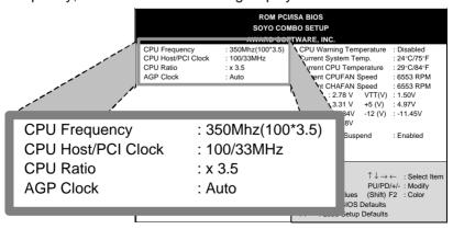
Available [CPU Frequency] settings on your SY-6BA+ Mainboard are detailed in the following table. If you set this field to [Manual], you are then required to fill in the next two consecutive fields: (1) the CPU Host/PCI Clock, and (2) the CPU Ratio.
