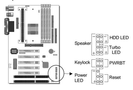
Plug the computer case's front panel devices to the corresponding headers on the mainboard.
