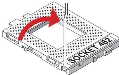
2. Take note of the red circle as below picture. While inserting the CPU into the socket, you can find out there is a definite pin orientation for CPU and socket.
