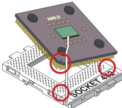
3. Make sure that the CPU position in the socket tightly, and then put the lever down to complete the CPU installation.
