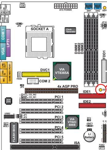
**NOTICE :** When LED “ZD1” light is on, meaning that 3.3V is operating and flowing into DIMM slots, please do not add or remove memory modules .
