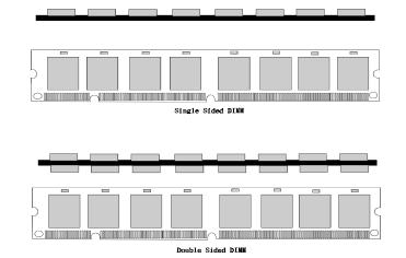
1. The DIMM socket has a "Plastic Safety Tab" and the DIMM memory module has an asymmetrical notch", so the DIMM memory module can only fit into the slot in one direction.
