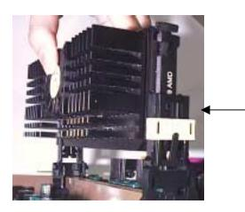
The correct direction to insert the Heat Sink and CPU into the Heat Sink Support Frame should allow you to easily insert them.
