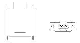
The serial ports on this system have two 9-pin connectors. Some older computer systems and peripherals used to be equipped with only one 25-pin connector. Should you need to connect your 9-pin serial port to an older 25-pin serial port, you can purchase a 9-to-25 pin adapter.
