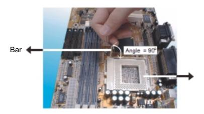
3. Locate Pin 1 in the socket and look for the cut edge in the CPU, match Pin 1 with the cut edge then insert the CPU. It should insert easily.
