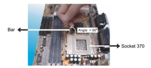
3. Locate Pin 1 in the socket and look for the cut edge in the CPU, match Pin 1 with the cut edge then insert the CPU. It should be inserted easily.
