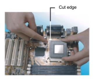
4. Press the lever down to lock the CPU into the socket.
