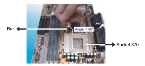
3. Locate Pin 1 in the socket and look for the cut edge in the CPU, match
