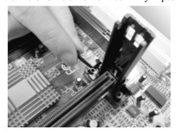
5. Slide the CPU slowly into Slot1 along the two sides of the CPU Retention.
