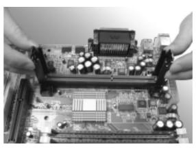
4. Ensure that the CPU Retention has been slotted all the way in, then screw the four plastic screws into the sockets on each side of Slot1 to make sure that the CPU Retention is fixed firmly in position.
