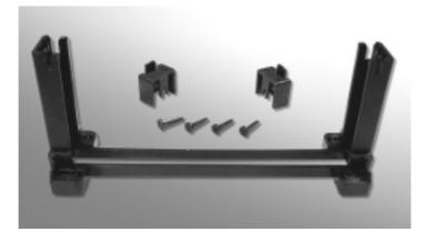
3. Once the above two steps have been completed, slot the CPU Retention into Slot1. Pull up the CPU stays on both side of the CPU Retention so they are horizontal, at an angle of 90°. Then the side of the CPU Retention with no mark on it and the side of Slot1 with the small rectangular tab should be on the same side.
