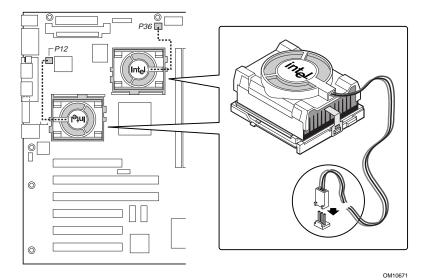
**8** After you have installed the processor(s), you must configure the speed jumpers.
