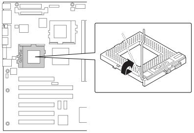
**3** Aligning the pins of the processor with the socket, insert the processor into the socket. Note what the processor speed is so you can set the jumpers correctly.
