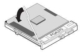
Place the fan heatsink on top of the processor.
