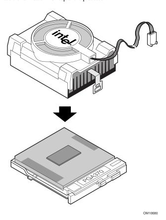
**6** Attach the fan heatsink clip to the processor socket. We recommend attaching the side away from the fan cable first. Then use a screw driver or other tool to attach the remaining side.
