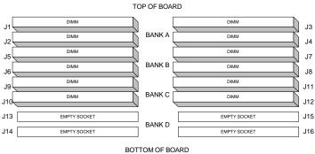
Figure 8.5: 4:1 Interleave with 12 DIMMS
