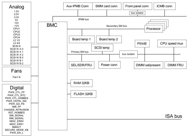
Figure 2.1: S450NX MP Server Management Block Diagram
