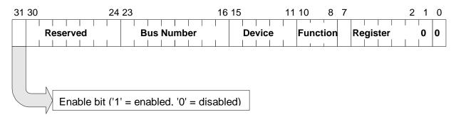
Figure 3.4: CONFIG\_ADDRESS Register
