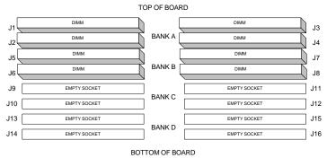
Figure 8.3: 4:1 Interleave with 8 DIMMS
