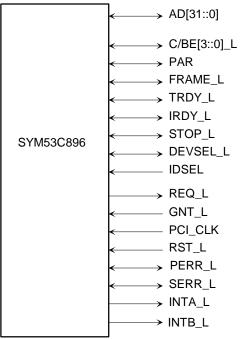
Figure 1.6: Embedded Wide SCSI PCI Signals
