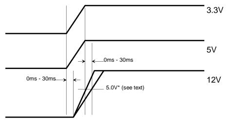
Figure 5.1: DC Voltage Sequencing
