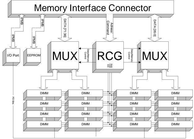
Figure 8.1: S450NX MP Server Memory Module Block Diagram
