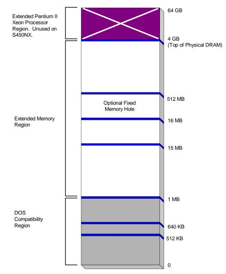
Figure 3.1: Pentium II® Xeon<sup>TM</sup> Slot 2 processor memory address space
