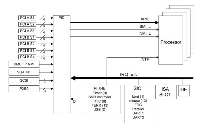
Figure 1.10: S450NX MP Server Baseboard Interrupt Diagram
