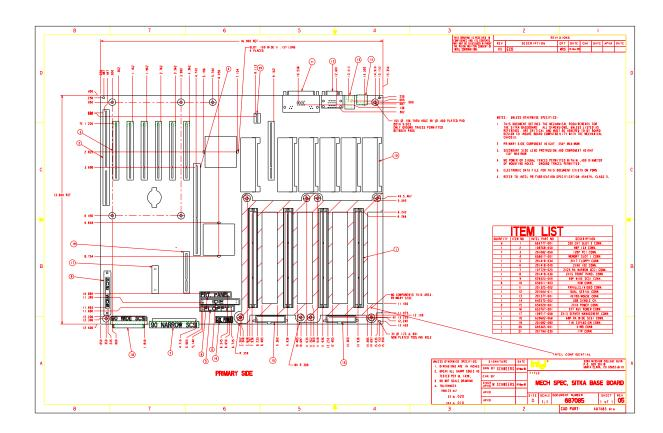
Figure 5.3: Baseboard Mechanical Diagram
