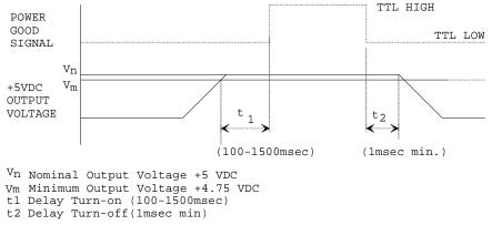
**Figure 5.2: Power Good Signal Characteristics**
