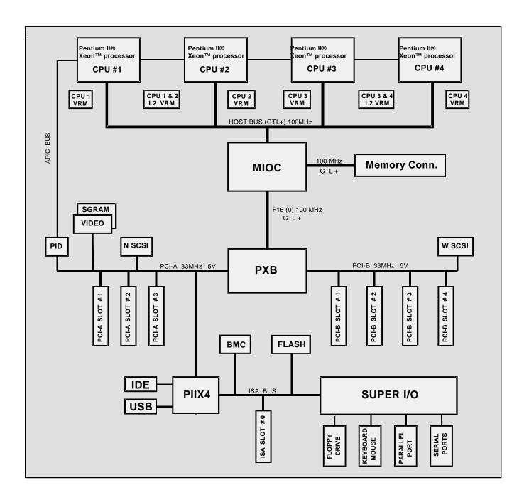
Figure 1.1: S450NX MP Server Functional Block Architecture
