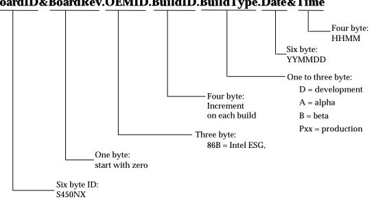
The figure below illustrates a standard 32-byte BIOS ID. BoardID&BoardRev.OEMID.BuildID.BuildType.Date&Time
