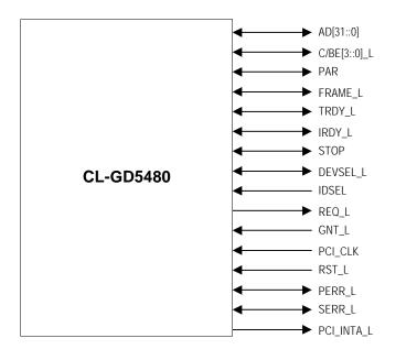
Figure 1.5: Video Controller PCI Signals
