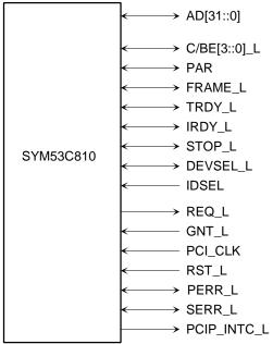
Figure 1.4: Embedded Narrow SCSI PCI Signals
