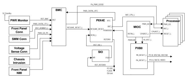
**Figure 1.8: Reset Flow Diagram**
