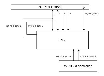
Figure 1.12: RAID configuration
