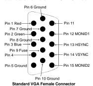
**Note:** If you want to disable the onboard VGA, short J17 and install a VGA card in J11 (PCI Slot1, Bus0.) An external PCI video card is supported in this slot only.
