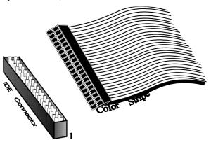
J10 is a 40-pin dual-inline shrouded connector that connects an ATA IDE drive to the primary onboard IDE connector. This motherboard supports IDE Mode 0 and LBA (Logical Block Address) mode, high capacity drives (over 528 MB), 32-bit data transfer, and fast IDE transfer. These IDE features are configured in Peripheral Setup in the AMIBIOS Setup utility.
