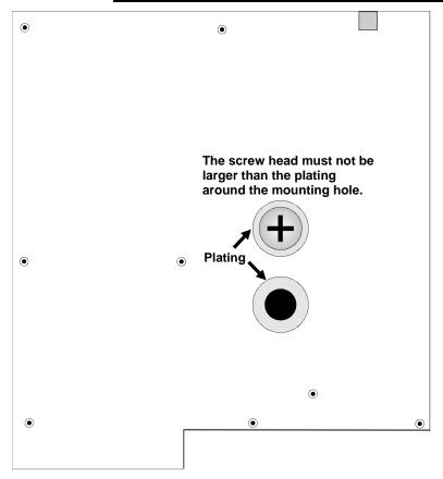
**Note:** The drawing above is only for illustration and does not show the exact position of the mounting holes.
