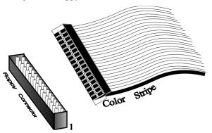
The motherboard supports up to two 720 KB, 1.44 MB, or 2.88 MB 3½" drives and 360 KB and 1.2 MB 5¼" drives. The connecting cable is a 34-pin ribbon connector with two 34-pin edge connectors for attaching the floppy disk drives. There is a small twist in the cable between the floppy connectors. The last (end) connector should be connected to floppy drive A: as shown below.
