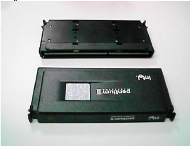
Figure 2: OEM Pentium® II Processor
