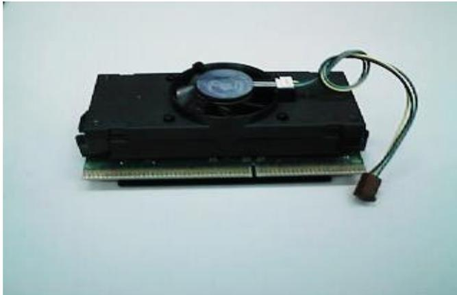
Figure 3: OEM Pentium® III Processor
