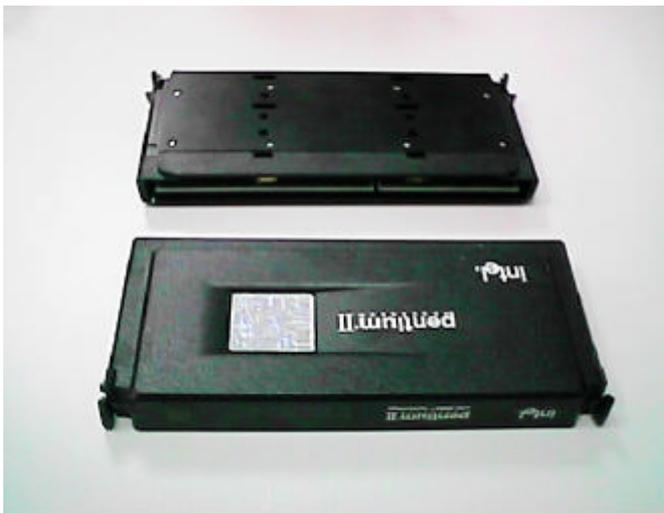
Figure 2:OEM Pentium® II Processor
