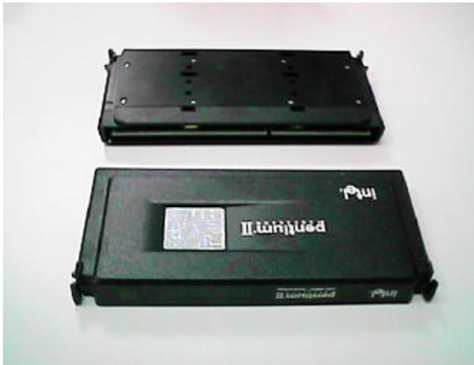
Figure 2:OEM Pentium® II Processor
