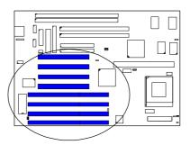
This section describes how to connect an expansion card to one of your system's expansion slots. Expansion cards are printed circuit boards that, when connected to the mainboard, increase the capabilities of your system. For example, expansion cards can provide video and sound capabilities.
