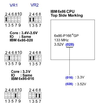
Core: 2.8V IO: 3.3V IBM: 6x86L \*
