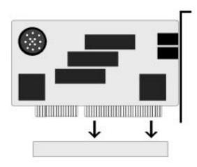
Figure 3-3: Installing an ISA Card
