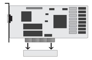
Figure 3-2: Installing a PCI Card
