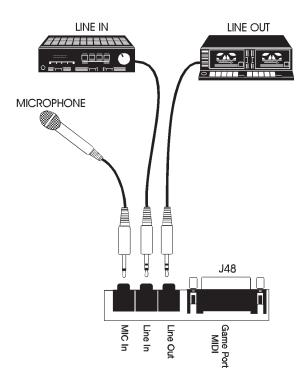
Figure 3-4: Connecting External Sound Devices
