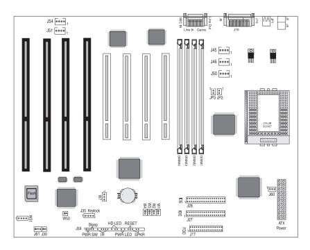
Figure 2-1: Invader ATX System Board
