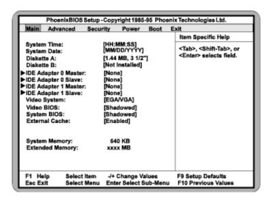
Figure 4-2: CMOS Main Screen
