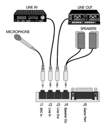
Figure 3-4: Connecting External Sound Devices
