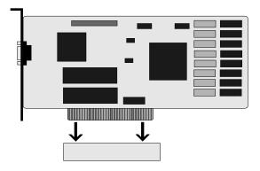
Figure 3-2: Installing a PCI Card
