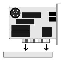
Figure 3-3: Installing an ISA Peripheral Card
