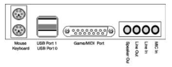
Figure 2.2: M55Hi-Plus Back Panel Connections
