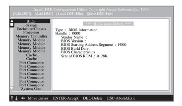
The four menus located on top of the DMI Configuration Utility screen are Edit DMI, Add DMI, Load DMI File and Save DMI File. Use the  $\leftarrow$  or  $\rightarrow$  (left or right) arrow keys to select a menu from the Menu bar:
