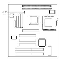
problems with PC-100 SDRAM DIMMs or you are using EDO / PC-66 SDRAM DIMMs, set the SDRAM clock according to the AGP clock (1-2 On).
