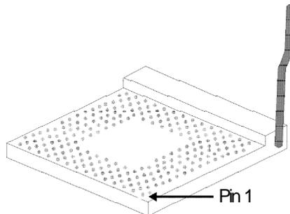
3. Position the CPU above the ZIF socket. Make sure pin 1 of the CPU is aligned with pin 1 of the socket. Lower the chip until the pins are inserted properly in their corresponding holes. Remember that very little force is needed to install the CPU. If the CPU is not easily inserted, verify whether or not pin 1 of the CPU is aligned with pin 1 of the socket. Applying too much pressure can damage the CPU or the socket.
