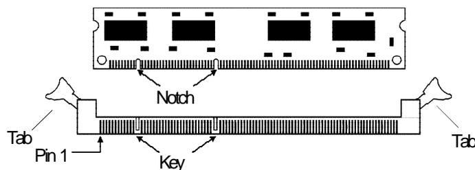
1. Pull the “tabs” which are at the ends of the socket to the side.
