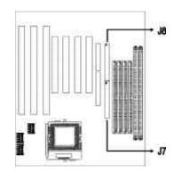
2 Install the other 40-pin header connector(s) into the device with the colored edge of the ribbon cable aligned with pin 1 of the drive edge connector(s).
