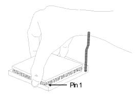
Positioning the CPU Above the ZIF Socket
