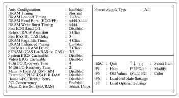
"Power-Supply Type" has been added into the Chipset Features Setup. The default is "AT" (for an AT power supply). If you are using an AT power supply and you set this field to "ATX", hardware reset will not function properly.
