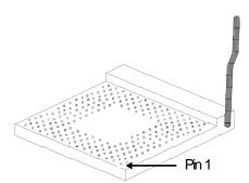
Position the CPU above the ZIF socket. Make sure pin 1 of the processor is aligned with pin 1 of the socket. Lower the chip until the pins are inserted properly in their corresponding holes. Remember that very little force is needed to install the processor. If the processor is not easily inserted, verify whether or not pin 1 of the processor is aligned with pin 1 of the socket. Applying too much pressure can damage the processor or the socket.
