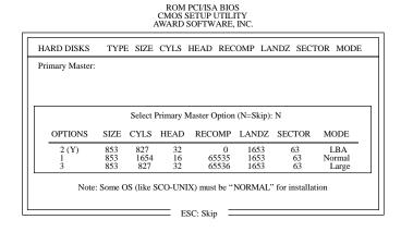
Enter your choice, and press <Enter> to accept the parameters or press <Esc> to abort. The parameters of the hard disk will be displayed in the Standard CMOS Setup.
