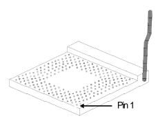
3. Position the processor above the ZIF socket. Make sure pin 1 of the processor is aligned with pin 1 of the socket. Lower the chip until the pins are inserted properly in their corresponding holes. Remember that very little force is needed to install the processor. If the processor is not easily inserted, verify whether or not pin 1 of the processor is aligned with pin 1 of the socket. Applying too much pressure can damage the processor or the socket.
