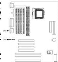
You may not use IrDA (CN4) and the COM 2 serial port (CN3) at the same time. If you are using the COM 2 serial port, set "UART 2 Mode" to Standard.
