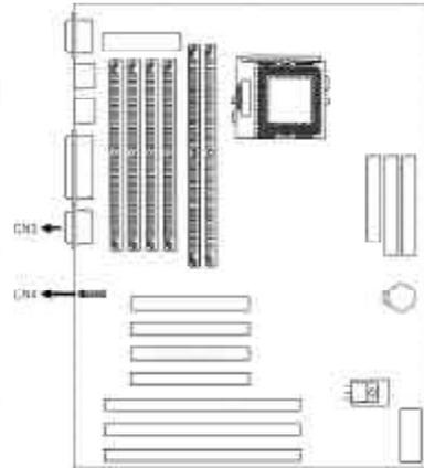
You may not use IrDA (CN4) and the COM 2 serial port (CN3) at the same time. If you are using the COM 2 serial port, set "UART 2 Mode" to Standard.
