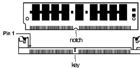
1. Position the SIMM above the socket with the “notch” in the module aligned with the “key” on the socket.
