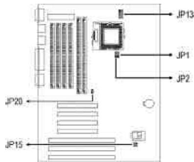
Jumper JP20 is used to set the external bus clock of your processor. Refer to the following pages for the external bus clock that corresponds to your processor and set this jumper accordingly. The clock generator will determine the external bus clock that must be sent to the processor through this setting.
