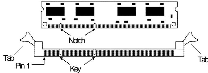
1. Pull the “tabs” which are at the ends of the socket to the side.
