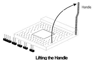
2 Once the lever is completely up, remove the old CPU carefully by lifting it straight out of the socket. You are now ready to insert the new CPU.
