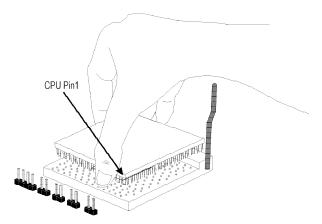
Positioning the CPU Above the ZIF Socket
