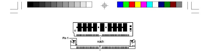
1. Position the SIMM above the socket with the "notch" in the module aligned with the "key" on the socket.
