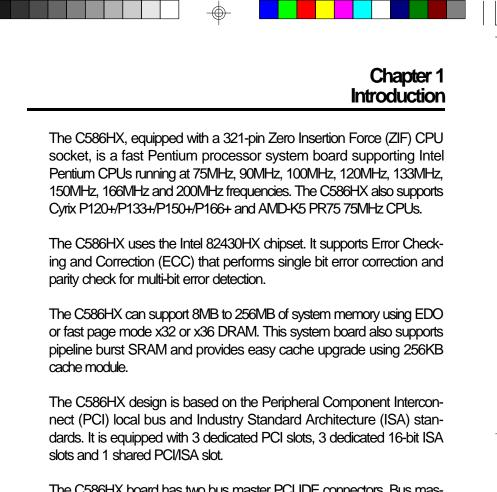
The C586HX board has two bus master PCI IDE connectors. Bus mastering reduces CPU use during disk transfer. This system board is also equipped with two NS16C550A-compatible serial ports, an SPP/ECP/ EPP parallel port, a floppy disk drive controller, one PS/2 mouse port, one PS/2 or AT keyboard connector and one IrDA header for wireless interface.
