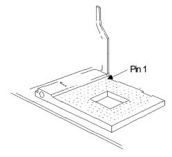
3. Position the CPU above the ZIF socket. Make sure pin 1 of the CPU is aligned with pin 1 of the socket. Lower the chip until the pins are inserted properly in their corresponding holes. Remember that very little force is needed to install the CPU. If the CPU is not easily inserted, verify whether or not pin 1 of the CPU is aligned with pin 1 of the socket. Applying too much pressure can damage the CPU or the socket.
