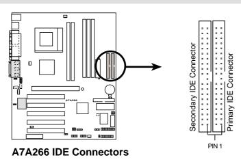
**NOTE:** Orient the red markings (usually zigzag) on the IDE ribbon cable to PIN 1.
