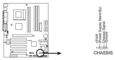
A7A266 Chassis Open Alarm Lead
