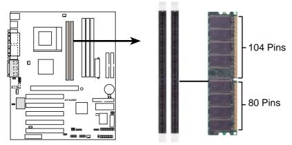
A7A266 184-Pin DDR DIMM Sockets
