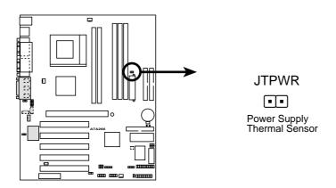
**A7A266 Thermal Sensor Connector**
