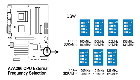
**WARNING!** Frequencies other than the recommended CPU bus frequencies are not guaranteed to be stable. Overclocking your processor is not recommended. It may result in a slower speed and premature wearing of the processor.
